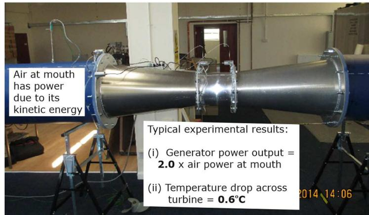
**Figure 14.** The first prediction was fulfilled in all of the power generating experiments that we carried out.
