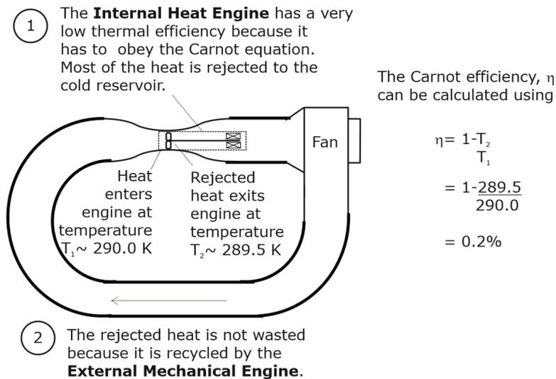
**Figure 2.** The internal heat engine must obey Carnot's equation and at the intended operating temperatures has an extremely low thermal efficiency. However by using an external mechanical engine to recycle the rejected heat, the external mechanical engine mimics the behaviour of an extremely efficient heat engine.
