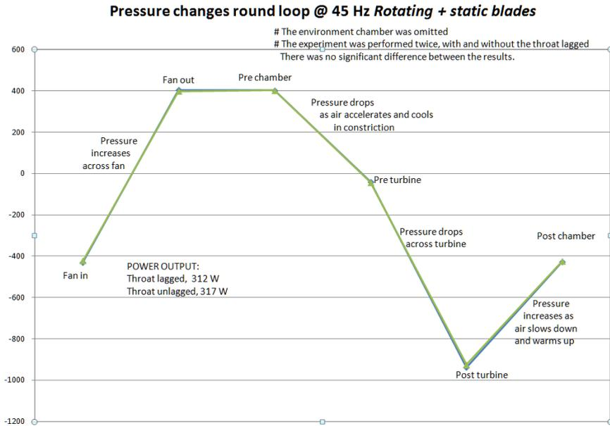
**Figure 25.** All of the closed loop experiments produced similar pressure changes around the loop.
