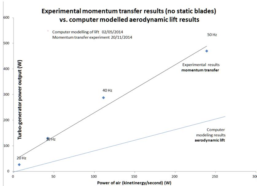
**Figure 23.** Momentum transfer delivered superior performance to aerodynamic lift.
