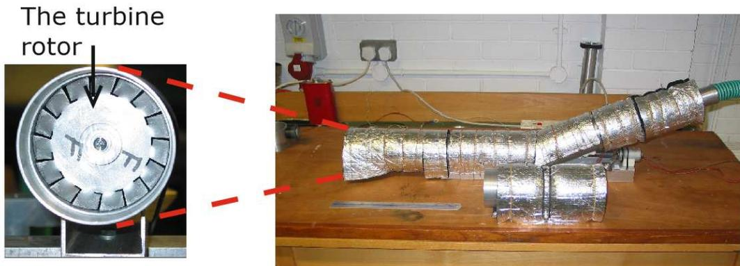
**Figure 3.** The test rig for the Lancaster University research 2009-10. The rig was designed to simulate the thermodynamic processes inside a hurricane.
