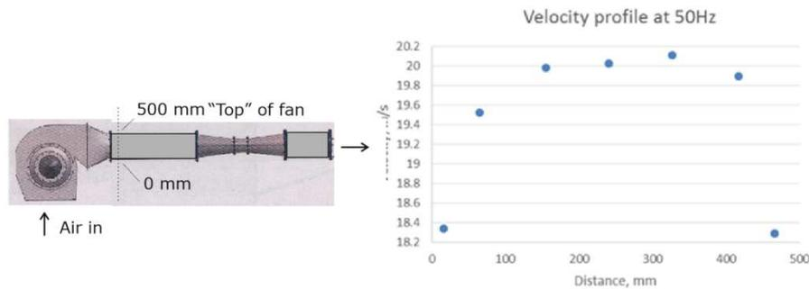
**Figure 21.** The profile indicated that when the fan was used to *push* the air through the constriction region, the flow rate was higher towards the top of the fan.
