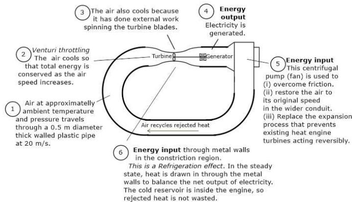
**Figure 10.** The Latent Power Turbine concept.
