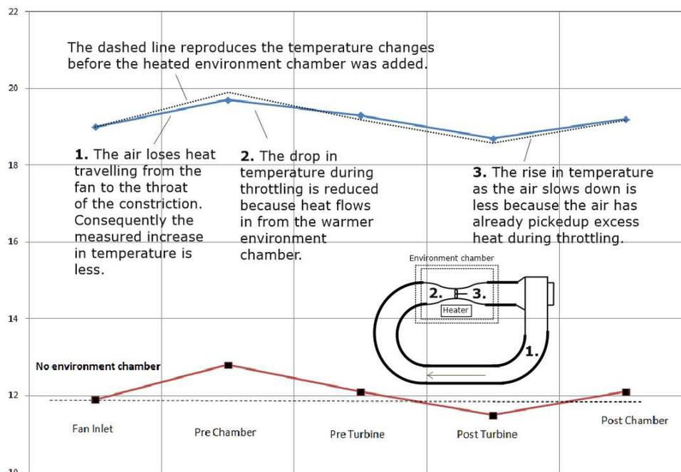
**Figure 19.** The small differences in temperature profiles are consistent with LP Turbine theory.
