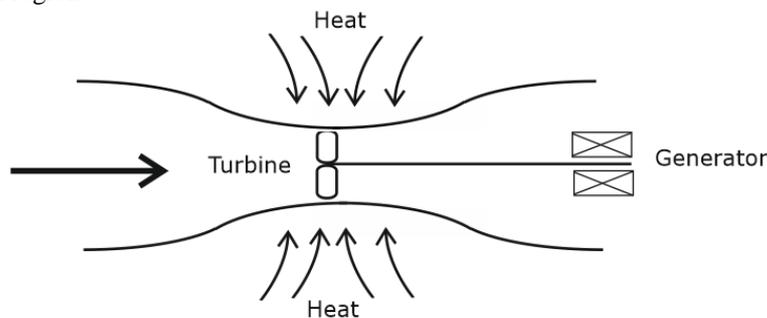
**Figure 9.** A heat engine inside a Venturi heat pump.
