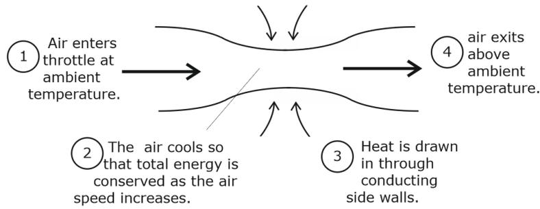
**Figure 8.** The Venturi heat pump effect.
