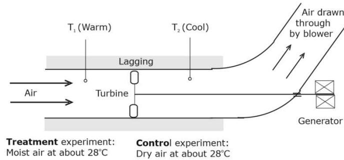
**Figure 5.** The turbine rotor throttled the air in the manner of a Venturi constriction. This meant that the dynamic air pressure dropped and the air transited the turbine blades at a lower temperature than 28°C. It was impractical to measure the air temperature at the location of the moving blades. So we estimated this by using the Bernoulli equation to estimate the drop in pressure and equating the gain in kinetic energy to a fall in internal energy.
