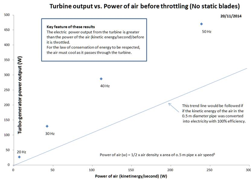
**Figure 13.** The four data points show the measured power output. They are consistently above the 100% trend line. This enables us to claim that,
