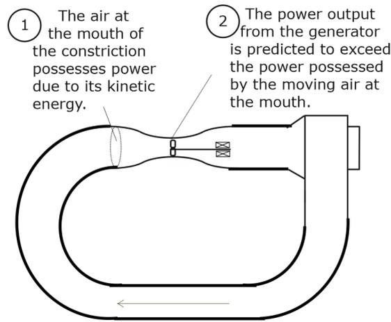
**Figure 12.** This prediction was fulfilled. But the turbo-generator only delivered about 10% of its theoretical maximum output. We assume that this was due to poor turbine design.
