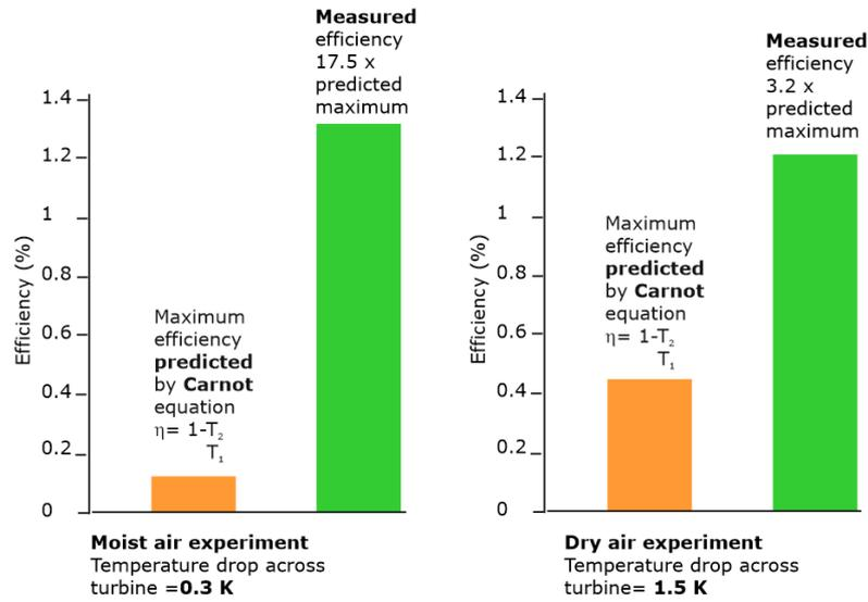
**Figure 6.** The dry air experiment also created an illusion that the Carnot equation had been violated.
