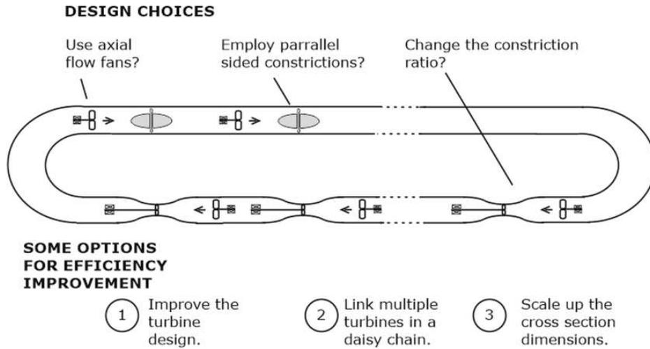
**Figure 28.** There is plenty of scope for improving the LP Turbine design.
