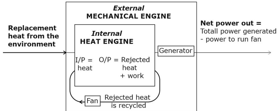
**Figure 11.** The internal heat engine must obey the Carnot equation and has a low thermal efficiency. But the external mechanical engine presents the *illusion* that it is a 100% thermally efficient heat engine.
