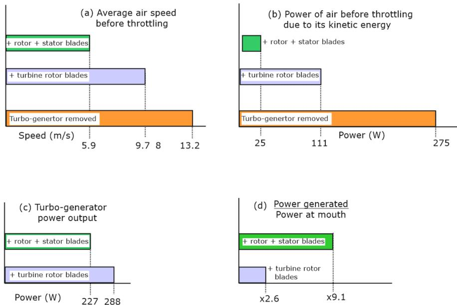
**Figure 27.** The environment chamber was removed and a fan speed of 40 Hz used for the above experiments.
