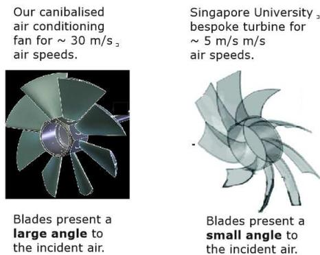
**Figure 20.** As for our work, the Singapore turbine was housed inside a parallel sided pipe.
