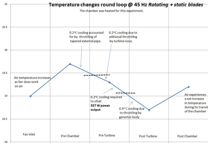
**Figure 17.** The expected thermal energy lost was calculated using values for the specific heat capacity of the air at constant pressure and the rate of mass flow.
