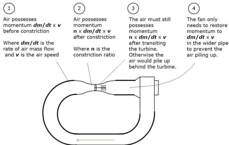
**Figure 24.** Strictly speaking, based on our Lancaster research, there is a slight drop in momentum after transiting the turbine because the air has cooled and its density has increased.
