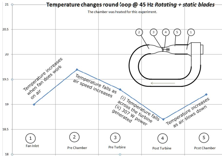
**Figure 16.** The Latent Power Turbine generated electricity and cooled the heated air inside the chamber.
