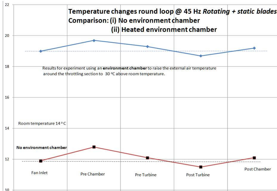
**Figure 18.** Even when the temperature gradient across the conduit walls was small, combined power generation and air cooling was still exhibited.
