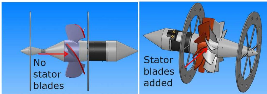
**Figure 26.** A second set of cannibalised air conditioning fan blades was used as stator blades. Their addition allowed the air to approach the rotor blades at an improved angle of attack.
